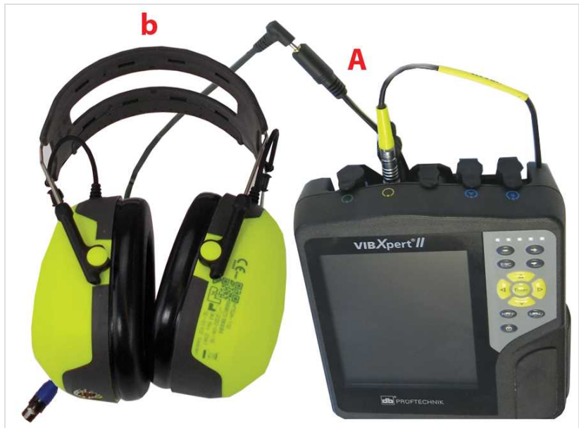
Mono headphones (b) attached to VIBXPERT II via the sensor cable VIB 6.675 (A)
